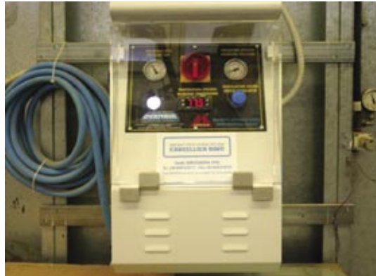
5 - The Top Spray module: it heats the nitrogen and helps further improve the formation of the film.
