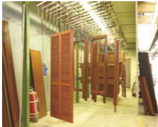
1 – Inside of the drying tunnel for the frames.
