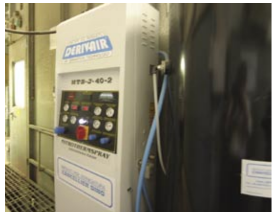
2 – The main module of the Nitrothermospray system (Cancellier Dino Impianti di Verniciatura). The nitrogen is produced in continuation through the selective permeation of the air through hollow fiber membranes.
